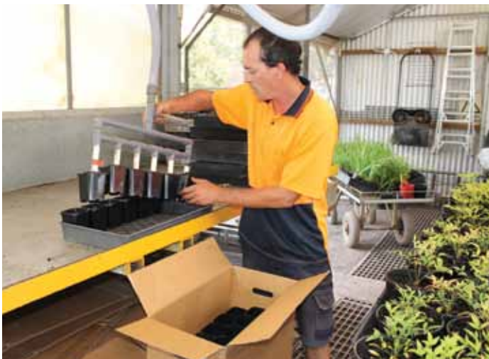
The 'Suckatron' lifts several pots simultaneously.
